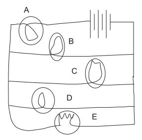
The sequence of how bright the bulbs are goes from A, which is the brightest, to D, then E, then B and finally C is the dimmest.
