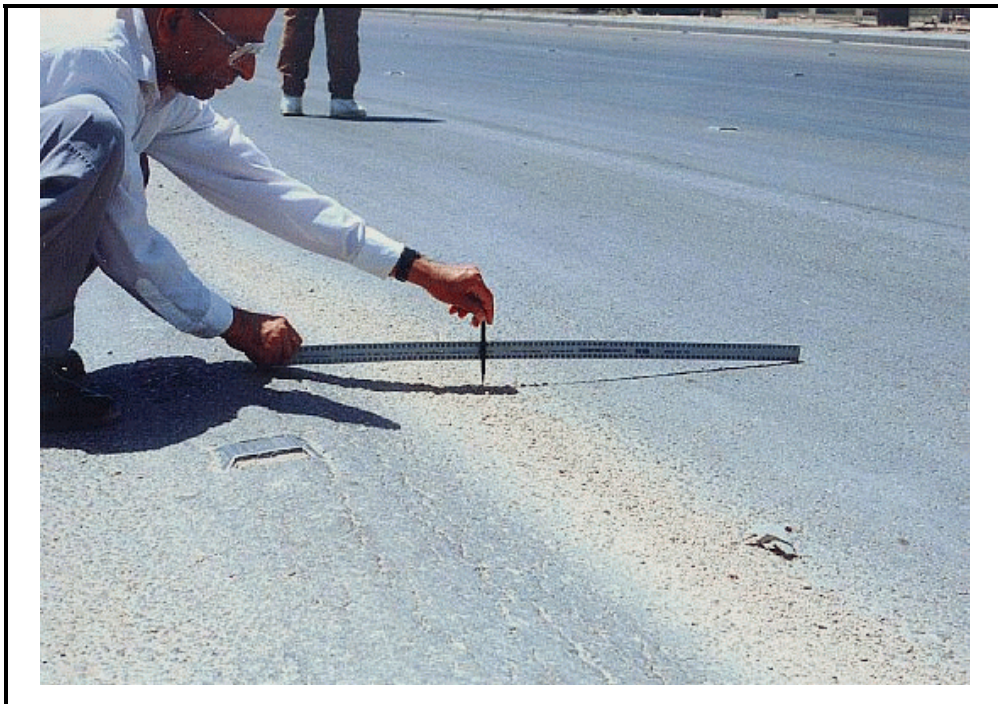
Photo A-11. Rutting in Flexible Pavement, High Severity
