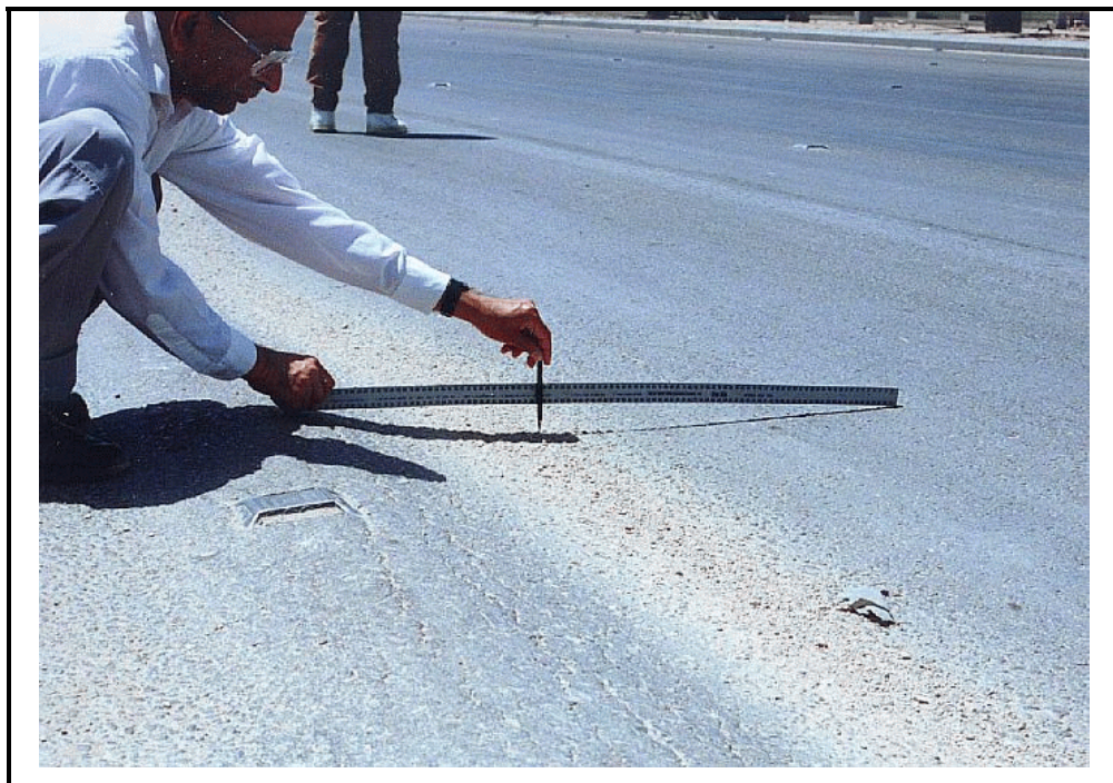
Photo B-10. Rutting in Composite Pavement, High Severity
