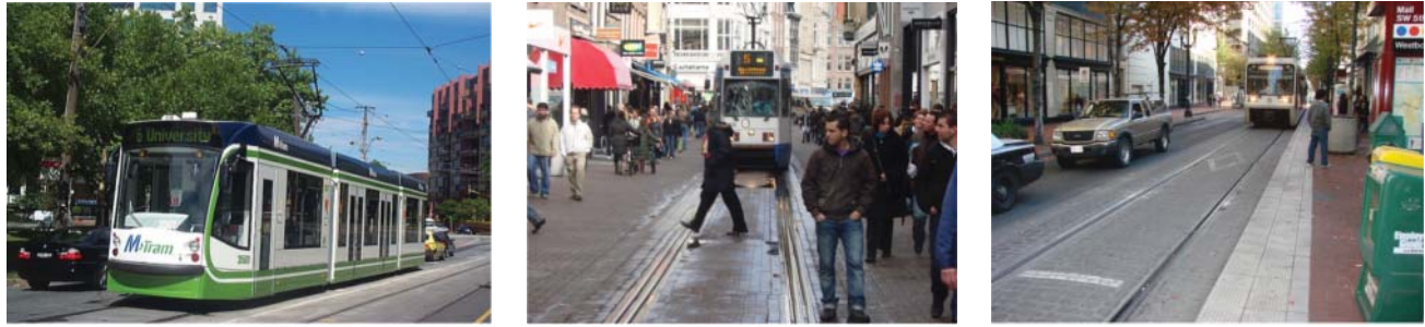
Figure 12-4. Mixed-Use Transit Right-of-Way, Category C. (a) Tram in Melbourne, Australia; (b) Streetcar in Amsterdam; (c) Light Rail in Portland, Oregon
