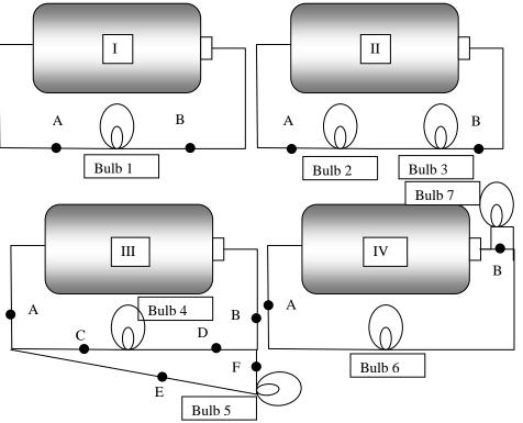
1) For each circuit, compare the flow of charge past point A with the flow of charge past B. Explain.
