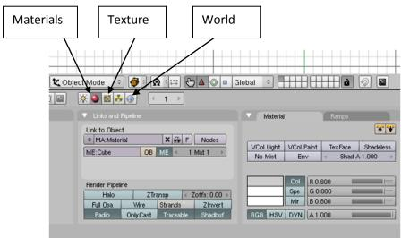
on the <u>shaders panel</u>. At the bottom of the shaders panel you see a number of settings: in particular if you look at one labeled **Spec** and the other labeled **Hard**. By adjusting hard, you change the size of the specular reflection. If you change the brightness of the specular reflection.
