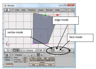
By default, the vertex button is selected in edit mode. Try selecting the edge mode and then click on an edge of the model. Try the face mode. See how these can ease the selection process?
