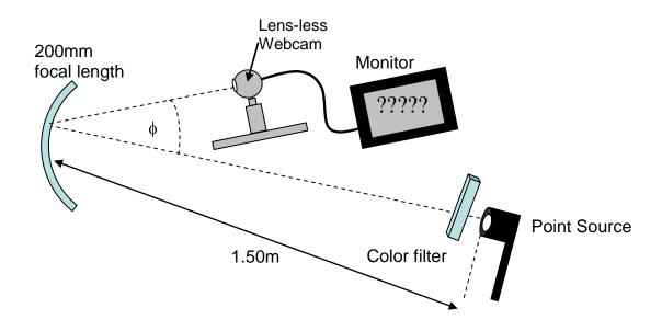
Adjust the camera position and record the distance from the mirror to the camera for the following circumstances. Make sure you readjust the focus each time. Note: you may have to adjust the shutter speed of the camera so that it doesn't saturate.
