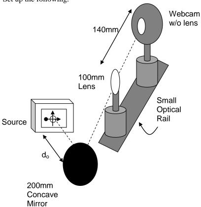
Fill out the following table and take pictures of the image (printing them) each time. "d<sub>i</sub>" is the distance from the concave mirror to where the image forms (as a result of the mirror). "x" is the distance from the 100mm focal length lens to where the image forms. To determine the magnification, find the ratio of the image size from the current set up to the image size from section I.
