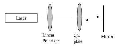
First turn the linear polarizer to 90° (where it should allow the most light to pass through). Reflect the laser light back towards the laser so that you can see the returning laser spot just to the side of the emission hole. Next, rotate the  $\lambda/4$  – plate to minimize the returning light power. What is the angle of the  $\lambda/4$  – plate?
