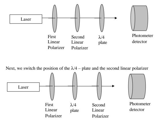
Predict how the light power reaching the photometer will change as a function of the <u>second</u> linear polarizer's angle. That is, make a plot of the transmitted laser beam power vs. the linear polarizer's angle.
