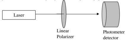
Rotate the linear polarizer to minimize the transmitted laser beam power. We will call this  $0^{\circ}$  and we will keep this definition throughout the rest of the investigation. NOTE: This designation more than likely does not agree with the values on the rotation stage. Rotate the linear polarizer by iterations of  $15^{\circ}$  until you rotate  $360^{\circ}$ . Complete the table and then using Excel plot your results.
