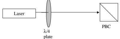
Rotate the  $\lambda/4$  – plate and describe what happens to the transmitted and reflected beams of light through the PBC as you turn the  $\lambda/4$  – plate.
