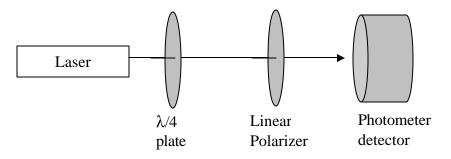
First turn the linear polarizer to its previous zero location (where it minimized the light from the laser). Next, rotate the  $\lambda/4$  – plate to minimized the light power at the photometer. We will call this 0° for the  $\lambda/4$  – plate and we will keep this definition throughout the rest of the investigation. NOTE: This designation more than likely does not agree with the values on the rotation stage.
