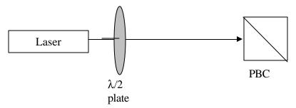
Rotate the  $\lambda/2$  – plate and describe what happens to the transmitted and reflected beams of light through the PBC as you turn the  $\lambda/2$  – plate. What do you think the  $\lambda/2$  – plate is doing to the polarization?
