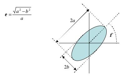
For elliptical polarization we can determine the tilt angle as well as the eccentricity by rotating a linear polarizer. The tilt angle is determined by angle at which the maximum amount of light passes through the linear polarizer. The eccentricity is found by
