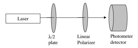
First turn the linear polarizer to its previous zero location (where it minimized the light from the laser). Next, rotate the  $\lambda/2$  – plate to minimized the light power at the photometer. We will call this 0° for the  $\lambda/2$  – plate and we will keep this definition throughout the rest of the investigation. NOTE: This designation more than likely does not agree with the values on the rotation stage.
