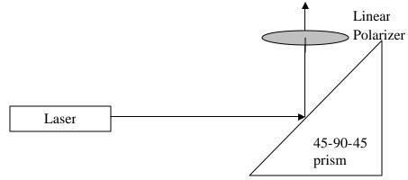
Keeping the same definition of  $0^{\circ}$  (regardless of whether it will now minimize the light in this new set up), predict the shape of a plot of the transmitted laser beam power (through the polarizer) vs. rotation angle of the polarizer.
