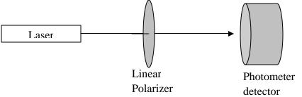
Rotate the linear polarizer to minimize the transmitted laser beam power. We will call this  $0^{\circ}$  and we will keep this definition throughout the rest of the investigation. NOTE: This designation more than likely does not agree with the values on the rotation stage.
