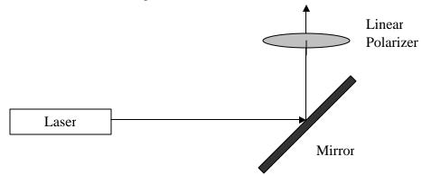
Keeping the same definition of  $0^{\circ}$  (regardless of whether it will now minimize the light in this set up), predict the shape of a plot of the transmitted laser beam power vs. rotation angle.
