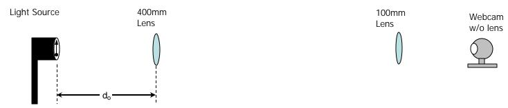
Predict what would happen if we remove the 100mm lens from the current set up. Could we get a focused image on the monitor by simply changing the webcam position?
