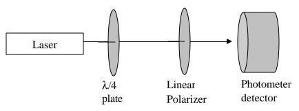
First turn the linear polarizer to its zero location (where it minimized the light from the laser). Next, rotate the  $\lambda/4$  – plate to minimized the light power at the photometer. We will call this 0° for the  $\lambda/4$  – plate and we will keep this definition throughout the rest of the investigation.
