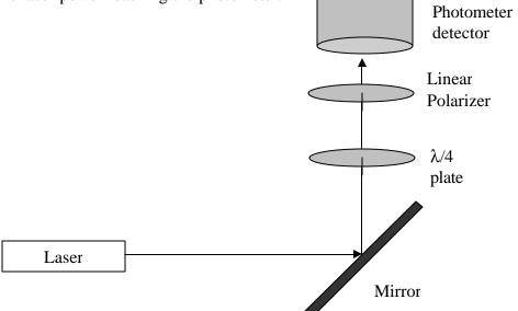
Predict the shape of a plot of the transmitted laser beam power vs. the linear polarizer's rotation angle.
