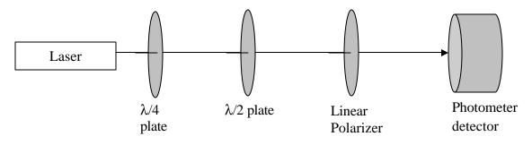
First turn the linear polarizer to its previous zero location (where it minimized the light from the laser). Next, rotate the first  $\lambda/4$  – plate to 22°. Finally, rotate the  $\lambda/2$  – plate to 0°. Predict how the light power reaching the photometer will change as a function of the linear polarizer's angle. That is, make a plot of the transmitted laser beam power vs. the linear polarizer's angle.
