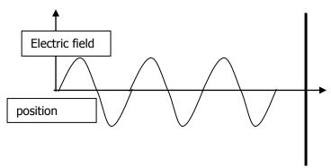
Consider the drawing above. We have the electric field of an EM wave traveling to the right. There is an antenna which is aligned with the electric field. What will happen to the wire as the wave travels past the wire?
