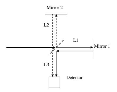
What is the relative phase of the two beams (one going to mirror 1 and one going to mirror 2) at the beam splitter?
