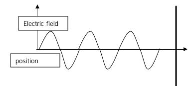
Consider the drawing above. We have the electric field of an EM wave traveling to the right. There is an antenna which is aligned with the electric field. What will happen to the wire as the wave travels past the wire?
