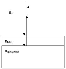
For an AR coating, what condition must we require for the phase difference of the two reflected beams?
