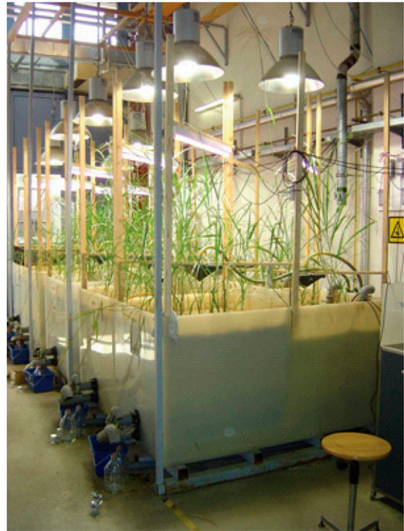
FIG. 3. Indoor pilot-scale constructed wetlands at the technical laboratory hall at the University of Natural Resources and Applied Life Sciences, Vienna (BOKU).
