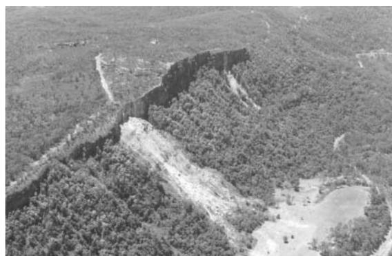
Fig. 2. Escarpment with large rock fall debris flow near Dombarton railway siding, 1974. Photo by Young.
