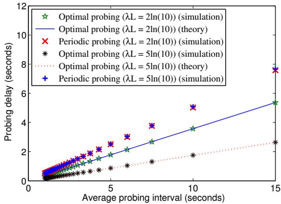
Fig. 7. Probing delay when a PU channel occupancy/vacancy distribution is a truncated exponential distribution ( $L = 1,500$  s and  $\Delta = 0.001$ ).
