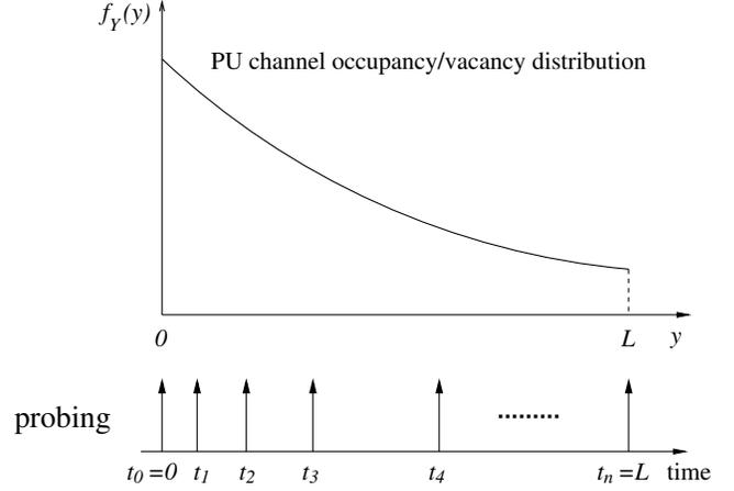
Fig. 5. An example of  $f_Y(y)$  and a spectrum-probing scheme.
