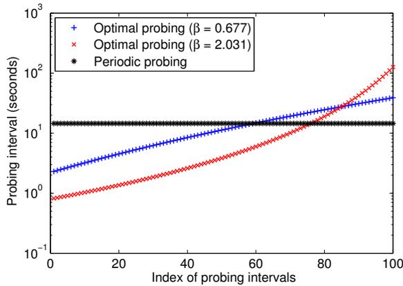
Fig. 8. Distribution of probing intervals when a PU channel occupancy/vacancy distribution is a truncated Pareto distribution ( $L = 1, 500$  s,  $y_m = 50$  s,  $n = 100$ , and  $\Delta = 0.001$ ).
