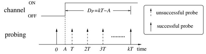
Fig. 2. Periodic probing with unreliable sensing.
