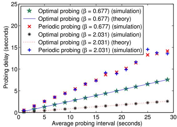
Fig. 9. Probing delay when a PU channel occupancy/vacancy distribution is a truncated Pareto distribution ( $L = 1, 500$  s,  $y_m = 50$  s, and  $\Delta = 0.001$ ).
