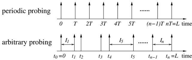
Fig. 3. A periodic-probing scheme versus an arbitrary probing scheme.
