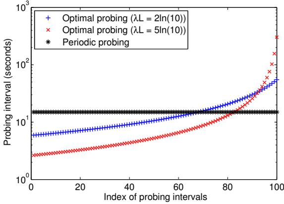
Fig. 6. Distribution of probing intervals when a PU channel occupancy/vacancy distribution is a truncated exponential distribution ( $L = 1,500$  s,  $n = 100$ , and  $\Delta = 0.001$ ).
