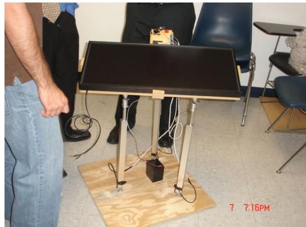
Figure 5: Solar tracker panel
