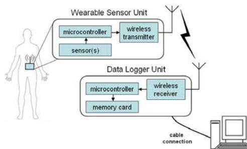
Figure 1- Overview of the wireless human movement monitoring system.
