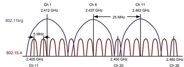
Figure 6- 802.11 and 802.15.4 channels in the 2.4GHz band.
