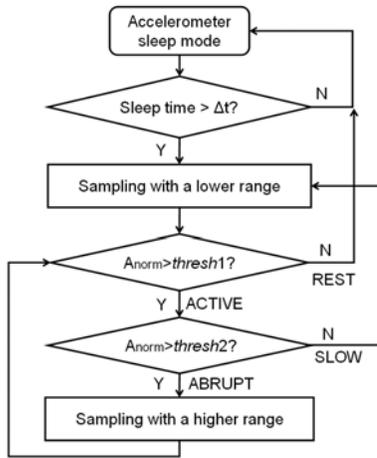
Figure 3- Workflow of the accelerometer.
