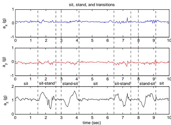
Figure 4- Acceleration measurement over three axes.
