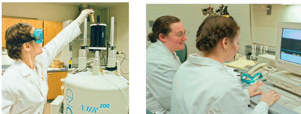
Figure 2. In the left-hand photo an NMR user is shown adding a sample to the carousel position 1. The standby position is ALWAYS position 9. In the right-hand picture the computer is used to acquire, process, and display NMR data.
