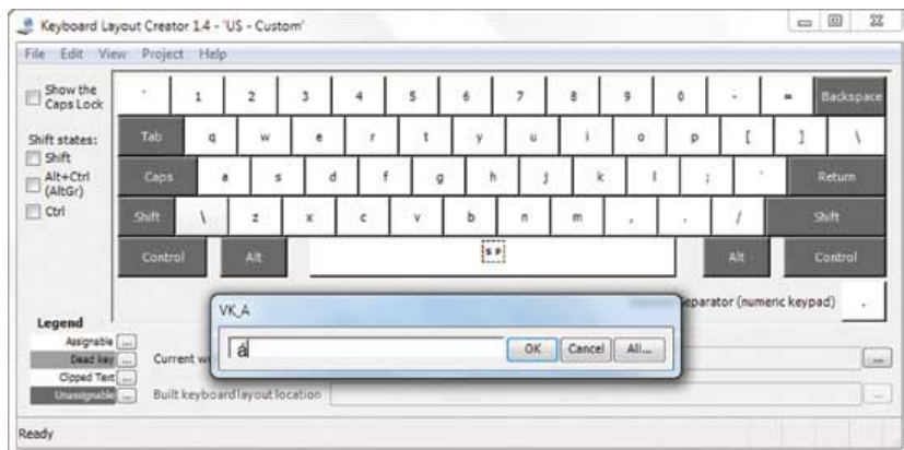
Figure 2 You can use the Microsoft Keyboard Layout Creator to create character accents.
