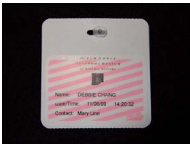
Figure 5.1: Time-activated Security Badge. A souvenir from my visit to NAL, this badge was printed at the time of my arrival. No stripes were at first apparent. Stripes appeared the day after my visit, invalidating the badge.
